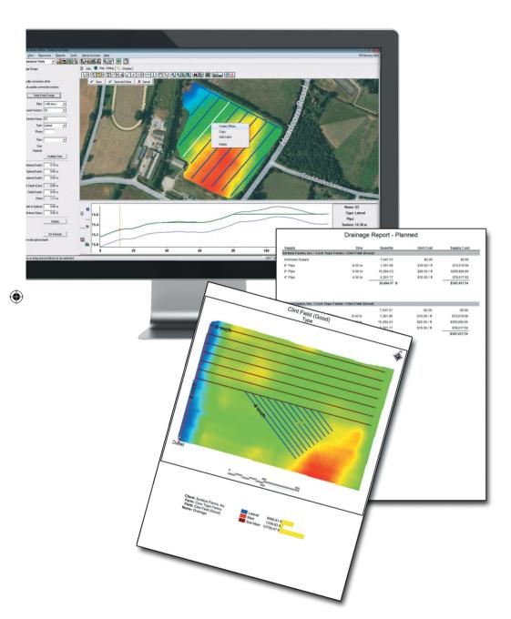
The Farm Works software - Surface is an analysis and design tool for use with Trimble agricultural drainage solution - WM-Drain -
